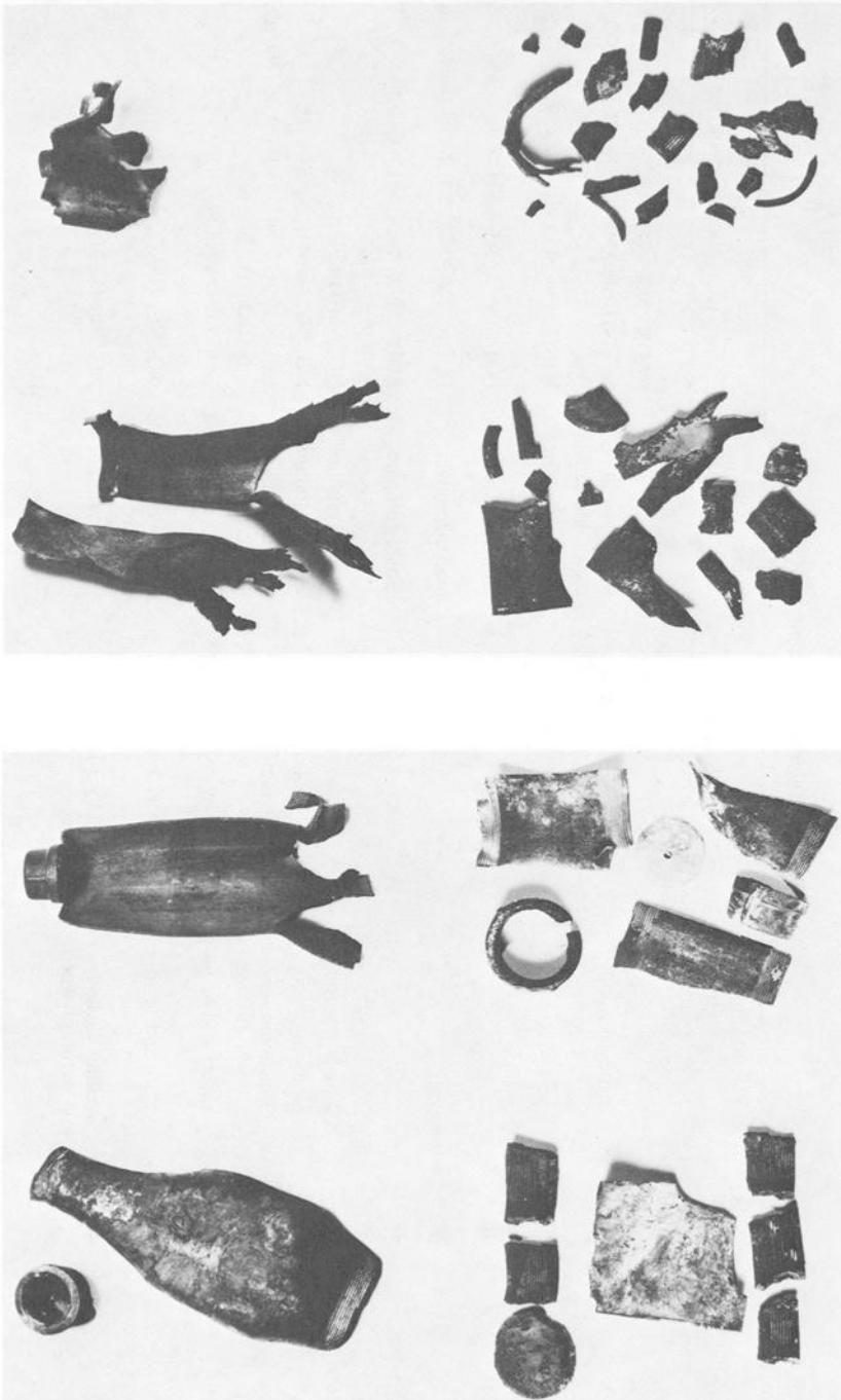
FIG. 4—Pipe bomb fragmentation by (left to right) black powder, single-base smokeless powder, double-base smokeless powder, and 40% dynamite: (top) 1 1/2-in. pipe and (bottom) 2 1/2-in. pipe.
